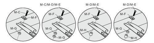
Note: Choose the appropriate screws, washers and spacers (if necessary) according to the type of screen.
