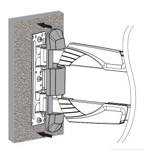
Install the decorative covers along the wall plate rail until they fit snuggly onto the wall plate.
