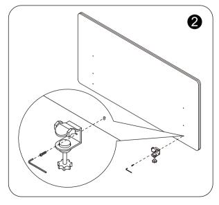
Insert screw through the clamp and into the panel.
