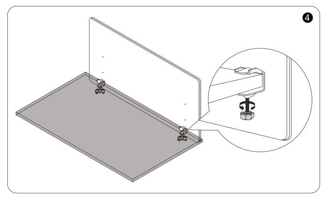
Rotate the screw to secure the panel to the edge of the desk.
