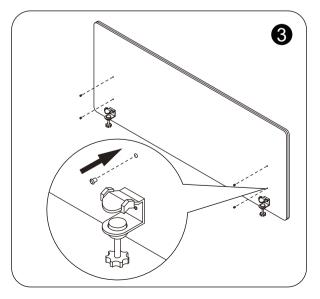
Insert hole plugs into the remaining holes until firm.
