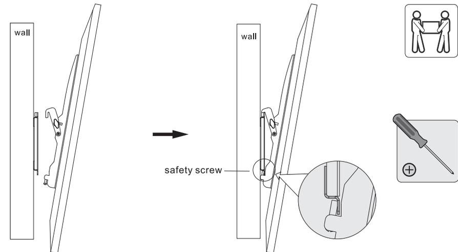
Hook the TV onto the upper ridge of the wall plate. Tighten the safety screws using a Phillips screwdriver to secure the TV to the lower ridge of the wall plate.
