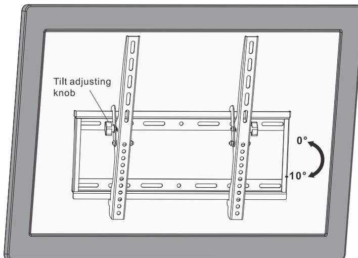
Use the tilt adjusting knobs to adjust your TV to the desired angle.
